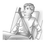
Buckle, position, and release the safety belt as described previously in this section. Make sure the shoulder portion of the belt is on the shoulder and not falling off of it. The belt should be close to, but not contacting, the neck. To remove and store the comfort guide, squeeze the belt edges together so that the safety belt can be removed from the guide. Slide the guide back into its storage pocket located on the side of the seat.
